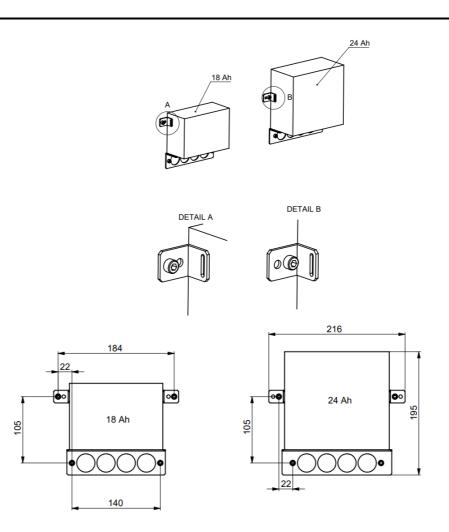
Material andESA-602-01-01 or ESA-602-01-02 depending on the battery typeDrawings:2x ESA-602-01-03<br/>Set of textile straps<br/>4x 1x Screw M5x30 DIN912<br/>4x Washer M5 DIN125A<br/>4x Self-locking Nut M5 DIN985
